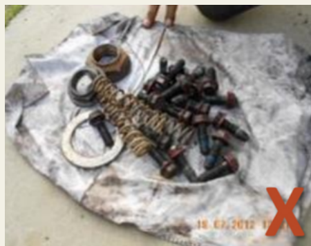
Examples of metal left inside a box that would have damaged the mulcher if un-detected
